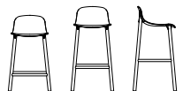
Stool with low back - wooden base L 45 P 53 H 82-92 cm W 17 3/8" D 20 7/8" H 32 2/8-36 2/8"
