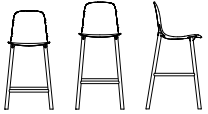
Stool with high back - aluminium base L 48 P 57 H 101-111 cm W 18 7/8" D 22 4/8" H 39 5/8-43 5/8"
